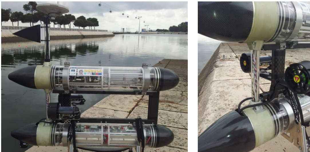
Fig. 3.1.1 a) A MEDUSA s vehicle with the new carbon fiber frame b) thrusters protective nozzle
