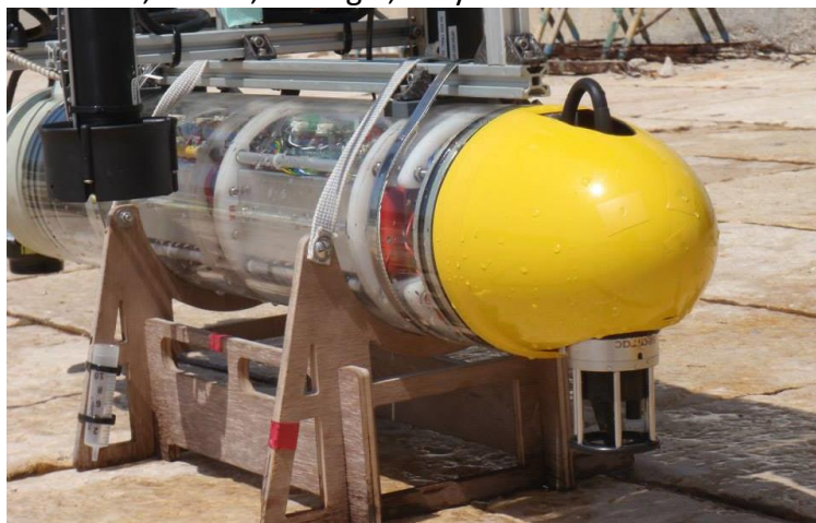
Fig. 3.1.2 Seatrac USBL mounted on Medusa Yellow
