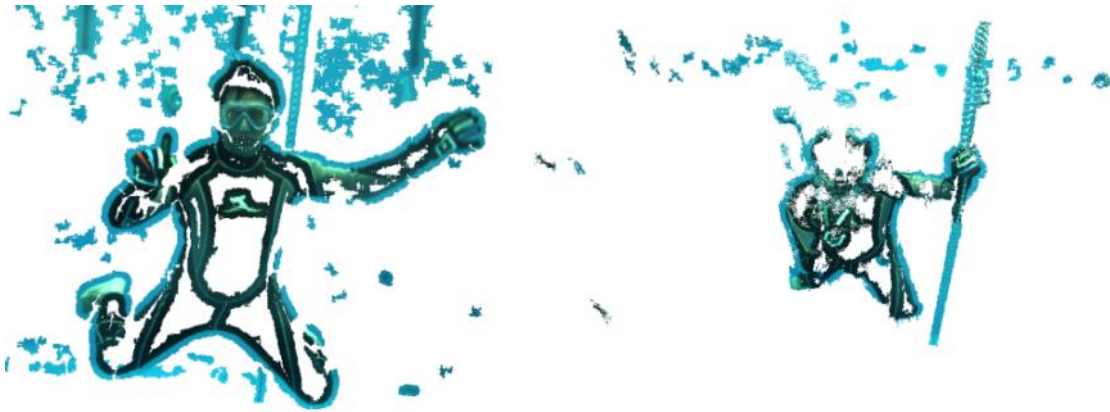
Resulting point clouds from the stereo images collected. Note that the contours of the diver are visible, but due to the lack of texture on the wetsuit, most of the diver is not properly reconstructed in 3D. This will be mitigated by a fused approach: A classifier will label diver pixels, and estimates will be filled in to the range image accordingly.
