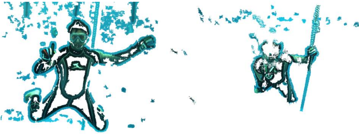
Figure 2.4.8: Resulting point clouds from the stereo images collected. Note that the contours of the diver are visible, but due to the lack of texture on the wetsuit, most of the diver is not properly reconstructed in 3D. This will be mitigated by a fused approach: A classifier will label diver pixels, and estimates will be filled in to the range image accordingly.
