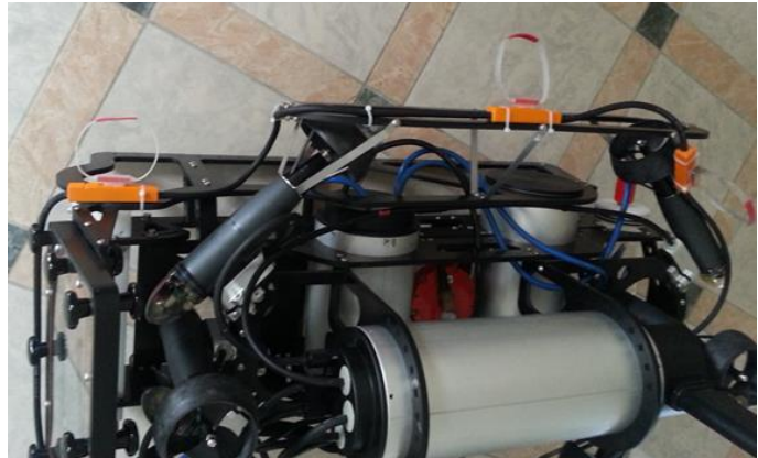
Figure 1.2.2. Haptic and reed kill switch
