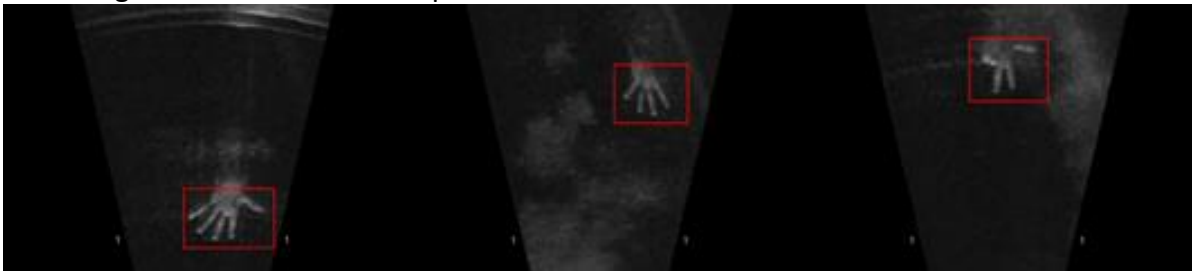
Three images of hand detection in sonar image using a cascade of boosted classifiers based on Haar-like features.
