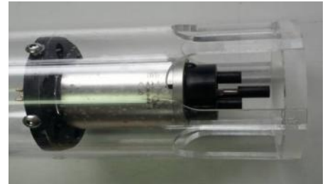
USBL with custom built cage
