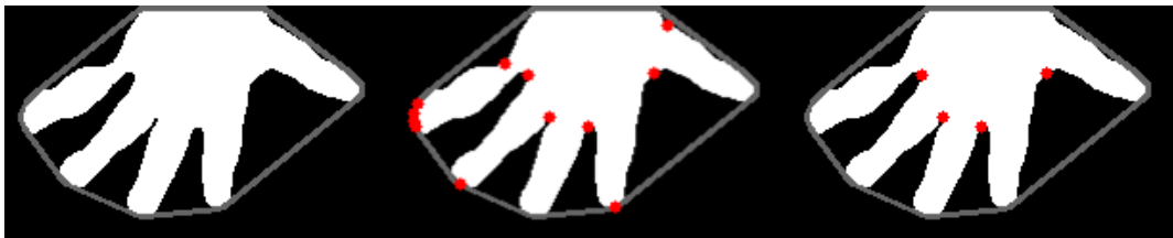
Fig. 2.6.5. Convex hull (left); all convexity defects (middle); filtered convexity defects (right)
