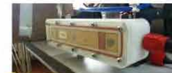
Stereo camera in an underwater casing mounted on BUDDY AUV
