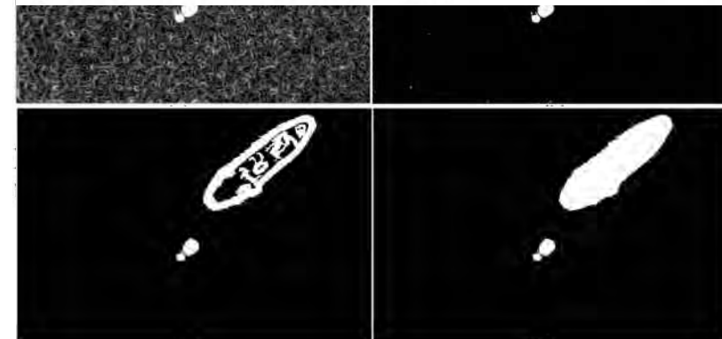
Figure 3. Before (a) and after (b) smoothing of the original image. The image is showing a large boat (length of 55m), a rigid-inflatable boat and a small buoy.
