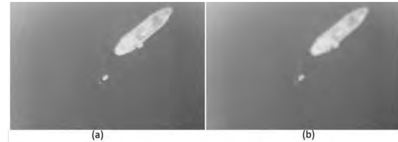
Figure 3. Before (a) and after (b) smoothing of the original image. The image is showing a large boat (length of 55m), a rigid-inflatable boat and a small buoy.
