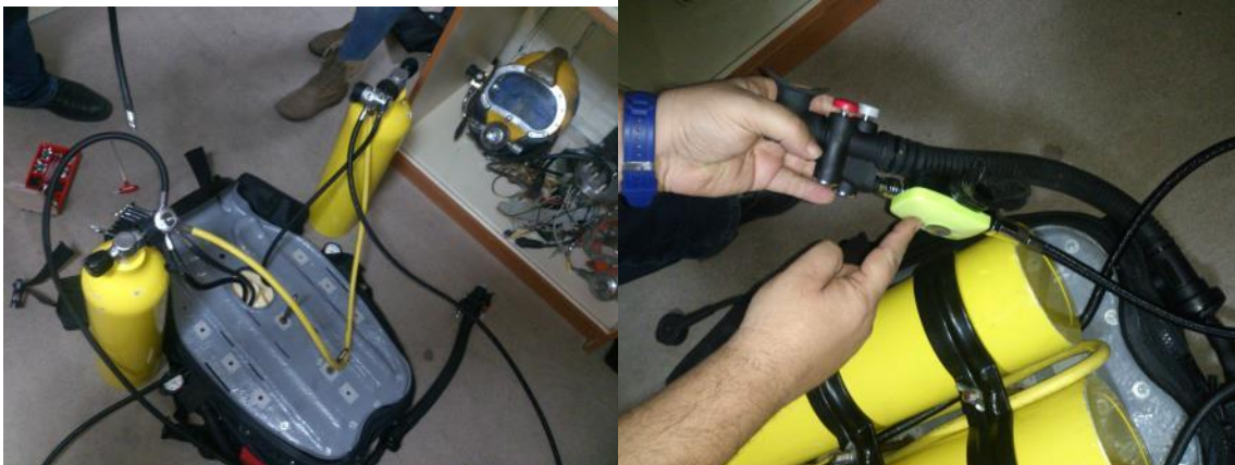
Figure 4 Dual tanks combined by the low pressure bridge (Picture on the left – yellow hose); all hoses are protected by the fiberglass case, spare regulator is attached to the BC hose (picture on the right yellow regulator).
