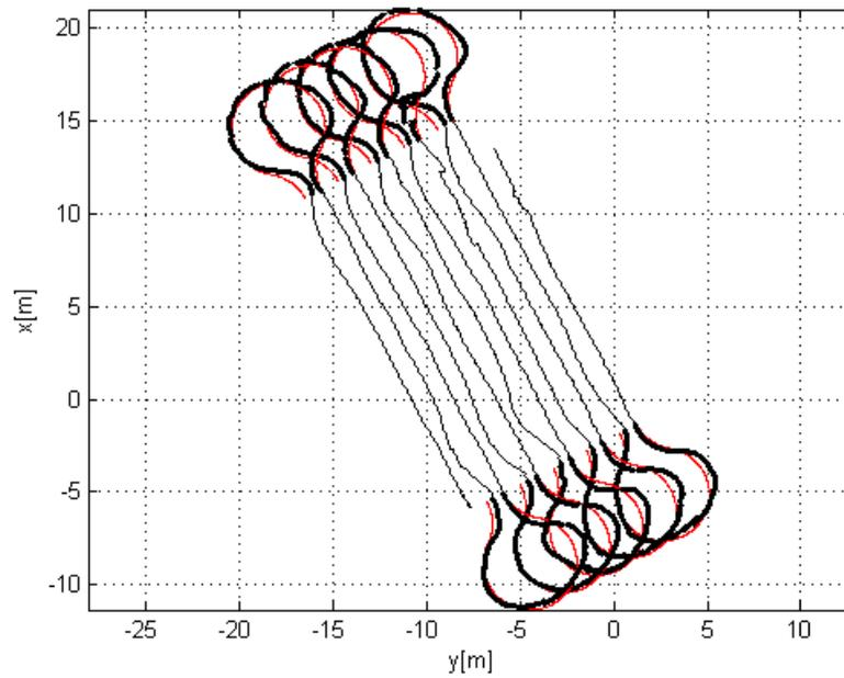
Fig. 2.10. Turn sections of the lawn-mower.
