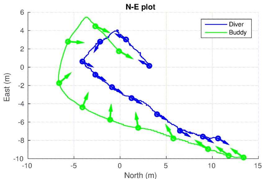
Fig. 4.21. Buddy overtaking surface platform during turns
