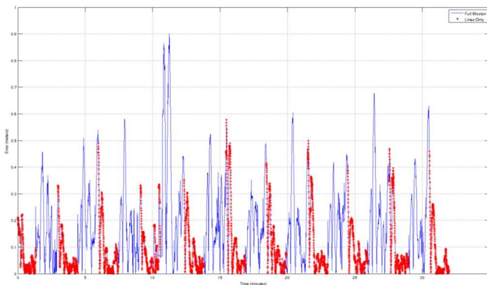
Fig. 2.8. Cross track error for the lines and full mission.
