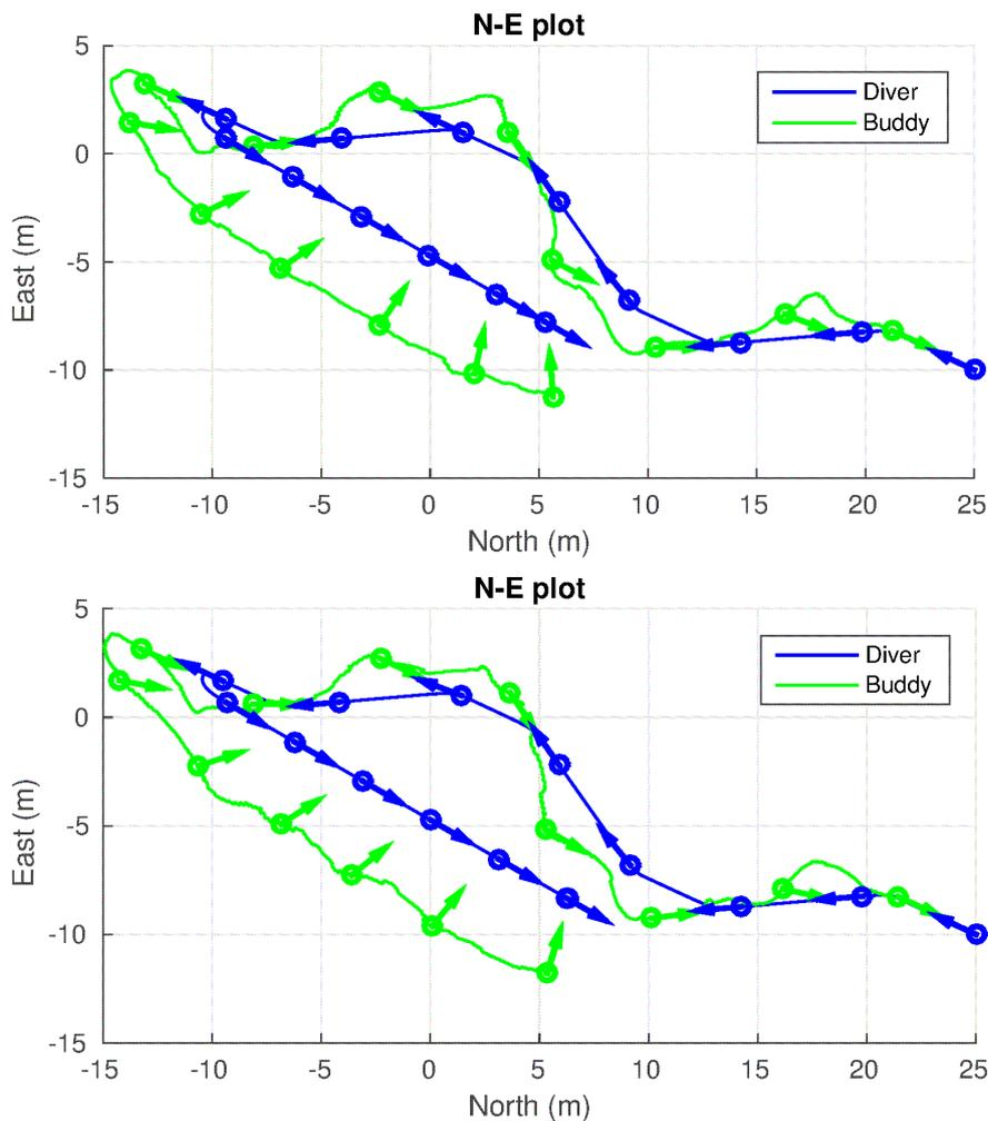
Fig. 4.17. North-East plot of diver tracking
