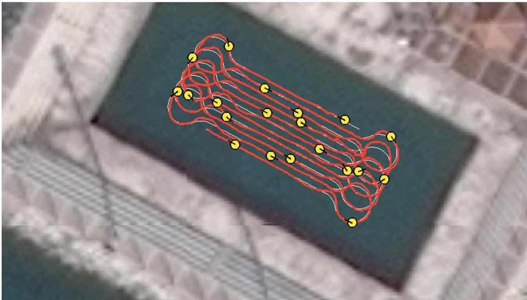
Fig. 2.7. Lawn-mower pattern mission inside a pool: nominal mission in white; vehicle path in red and vehicles pose the yellow circles.
