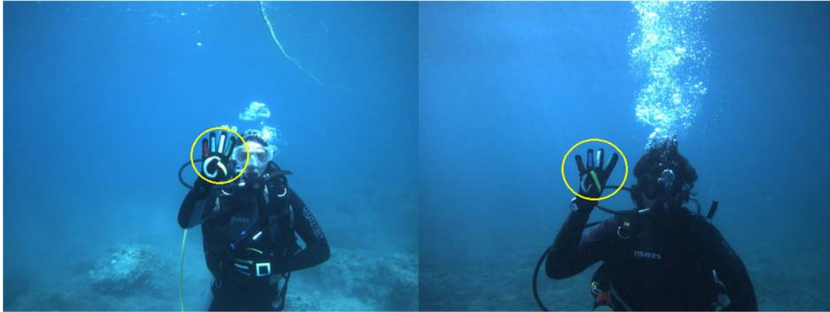
Figure 9. An example from field experiment: depending on the light conditions, colour markers on the gloves are differently interpreted.
