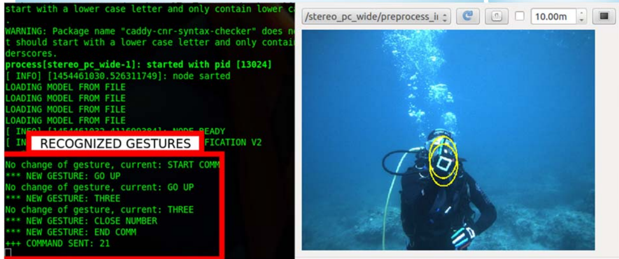
Figure 6. Classification system detecting hands and labelling individual gestures. If a "Start" and "End" communication gestures is received, the in-between symbols are checked by the syntax checker and sent to the AUV if correct.
