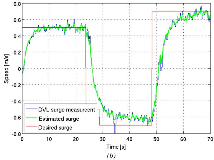
Fig. 3.1.3. (a) Heading response and (b) surge speed response of the Buddy vehicle
