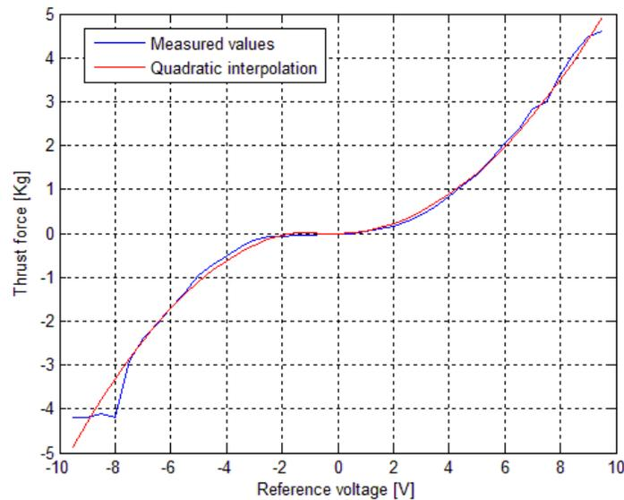
Fig. 3.2.2.3. e-URoPe AUV thruster force curve
