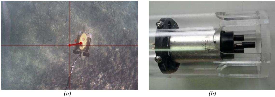
Fig. 3.2.2. (a) PlADyPos camera for tracking validation in shallow water and (b) custom made USBL cage
