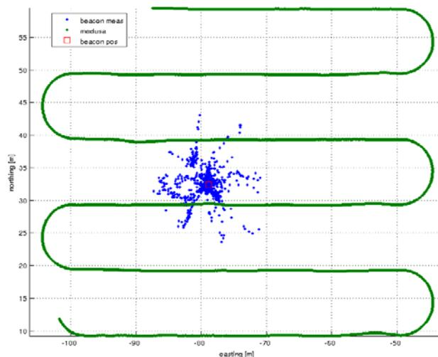
Fig 6.1.2 USBL fixes for a stationary beacon underwater
