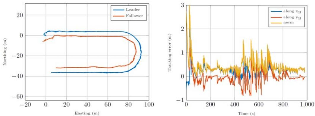
*Fig. 6.3.1. Leader Tracking System with AUV as leader.
