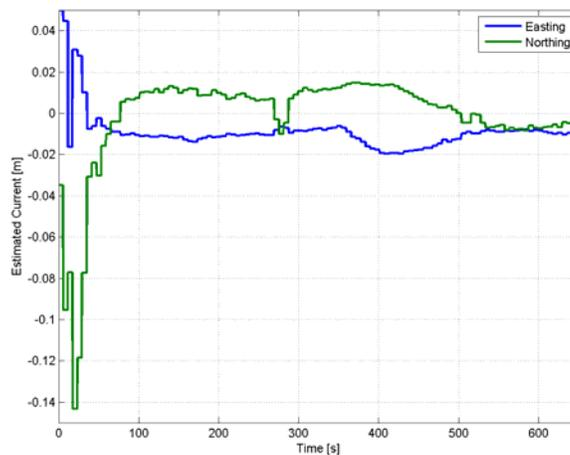
Fig. 6.2.3 Estimate of ocean current on-board the AUV
