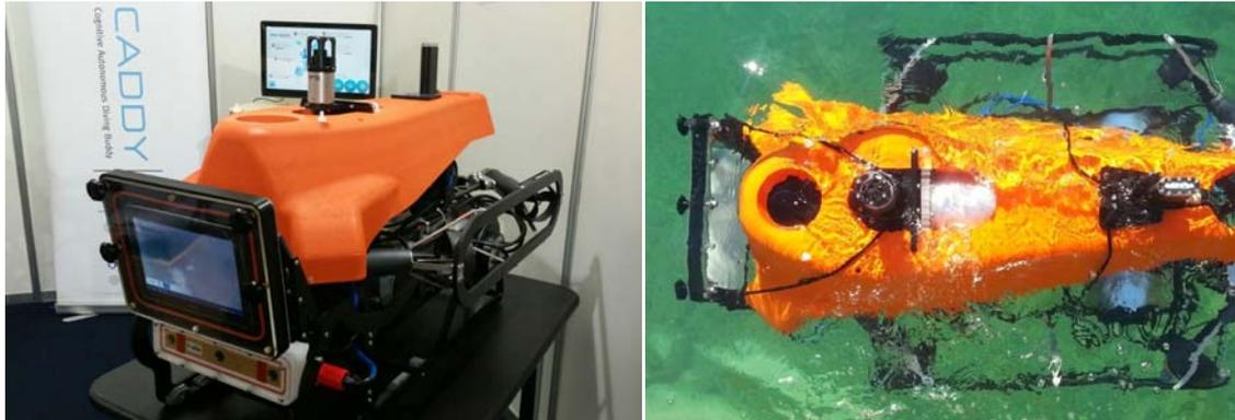
Fig. 3.1.1. The Buddy vehicle during assembly and in water
