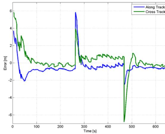
Fig. 6.2.2. Tracking error of the AUV
