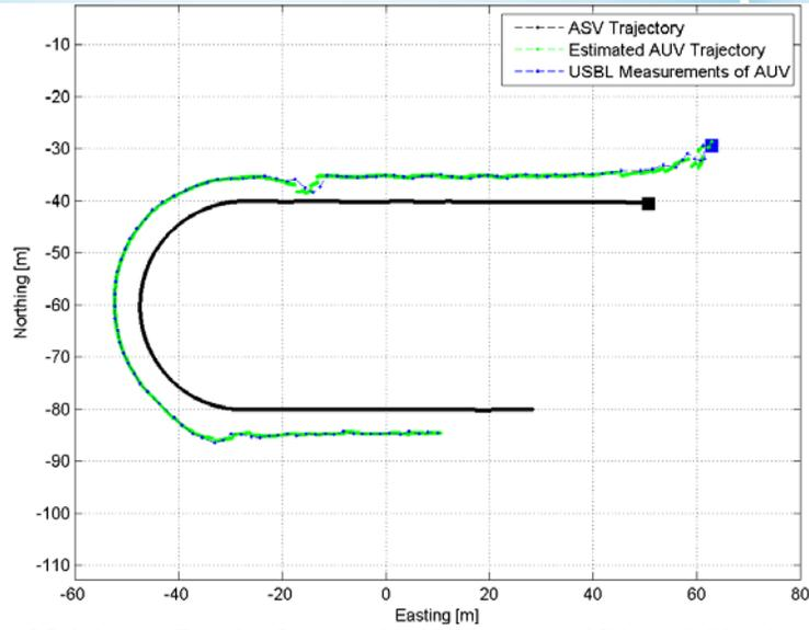
Fig. 6.2.1. Leader Tracking System with ASV as leader: ASV and AUV trajectories.
