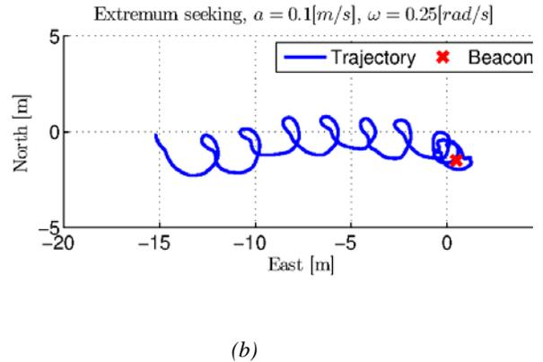
Fig. 3.2.3. PlaDyPos extremum-seeking tracking of the object with range-only measurements
