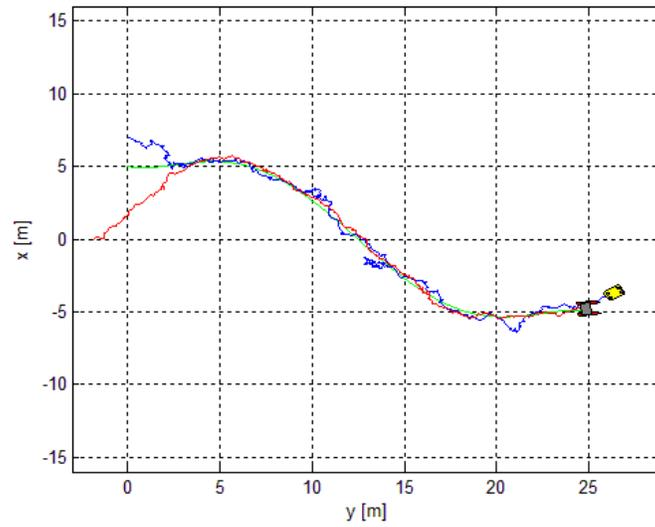
Fig. 5.5.3.4. Cooperation simulation corrupted by disturbances and communication delays
