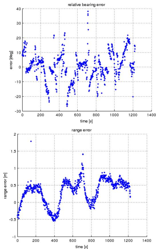
Fig 6.1.3 USBL Bearing and Range measurements against GPS positions
