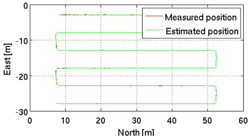
Fig. 3.2.3. PlaDyPos lawn-mower mission with GoTo primitives
