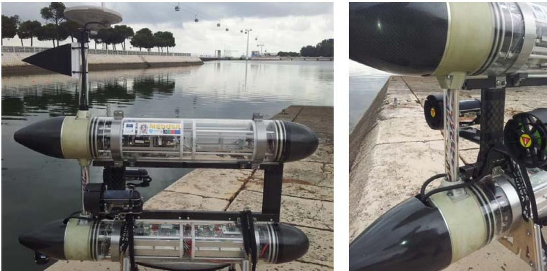
Fig. 3.1.2 a) A MEDUSA<sub>S</sub> vehicle with the new carbon fiber frame b) thrusters protective nozzle
