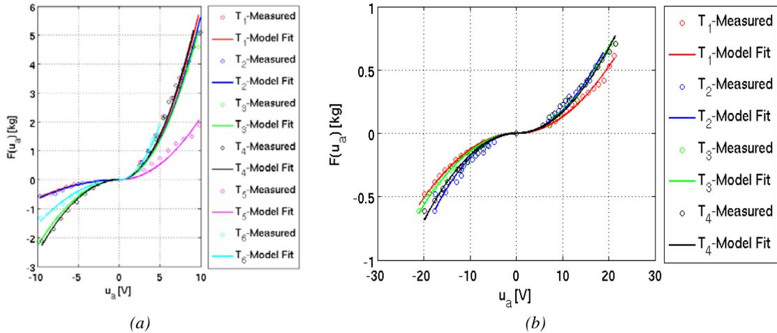
Fig. 3.1.2. Mapped and fitted thrust model ( $F=Kua|ua|$ ); (a) Buddy thrusters and (b) PlaDyPos thrusters
