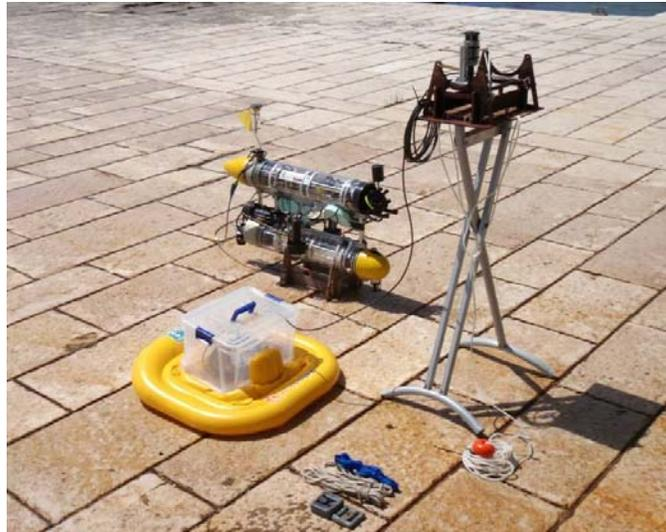
Fig 6.1.1 Experiment setup with the fixed beacon on the tripod and the USBL mounted on the MEDUSA<sub>s</sub>
