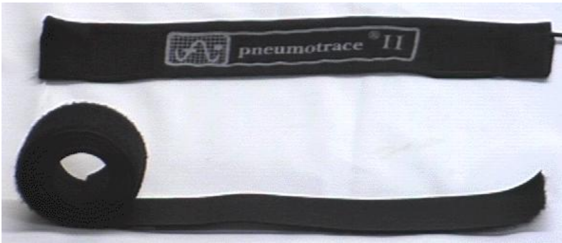
Fig 4.1. Breathing belt device
