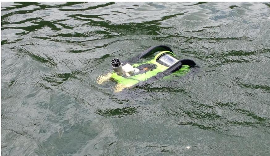
*Fig 3.4 – Seatrak modem deployed on Seabotix ROV*
