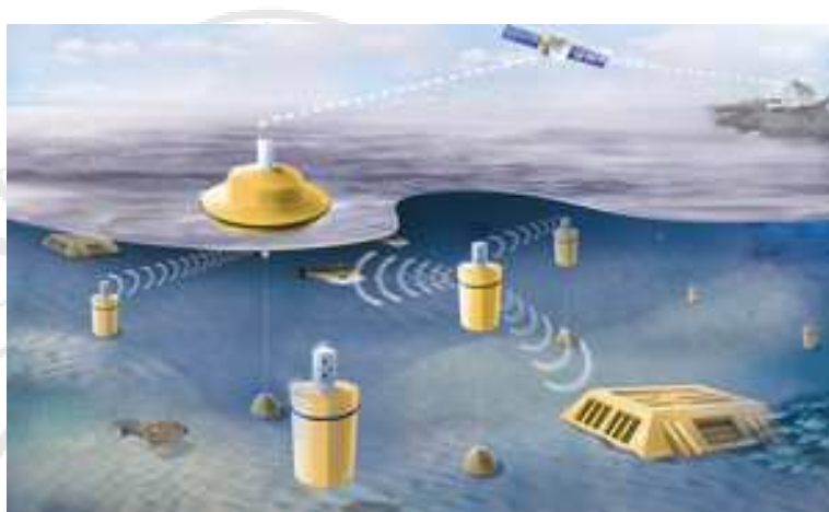
Fixed topology UW Acoustic Network
